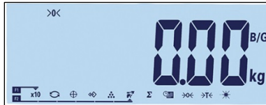
Figure 3-53: Animal Weighing, Scale Weight Returned to Zero
